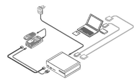
The FPS-8 flash prommer is used for heavy flashing. The sales pack product code is 0080321.
