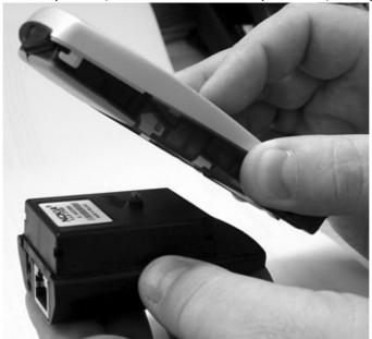
2 Align the battery connecter with the battery contacts of the adapter. Gently press the phone onto the adapter (see following picture).
