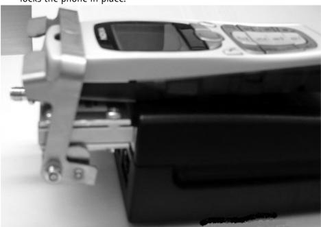
4 To remove the phone from the adapter, push the bottom connector end of the phone down to the hollow in the adapter. At the same time, push the upper end of the phone until it detaches from its place. Detach the phone in inverse order from installation.
