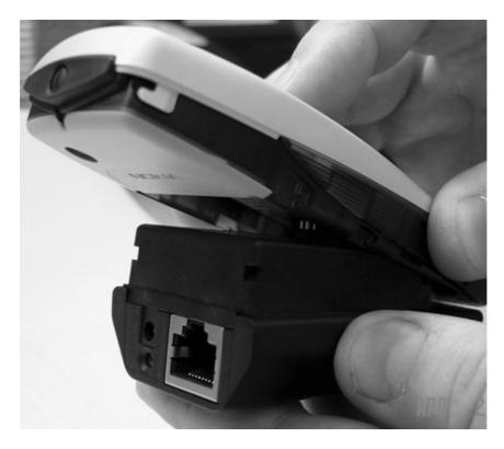
3 Press the upper end of the handset down onto the adapter until the battery tabs of the D-cover catch the adapter.
